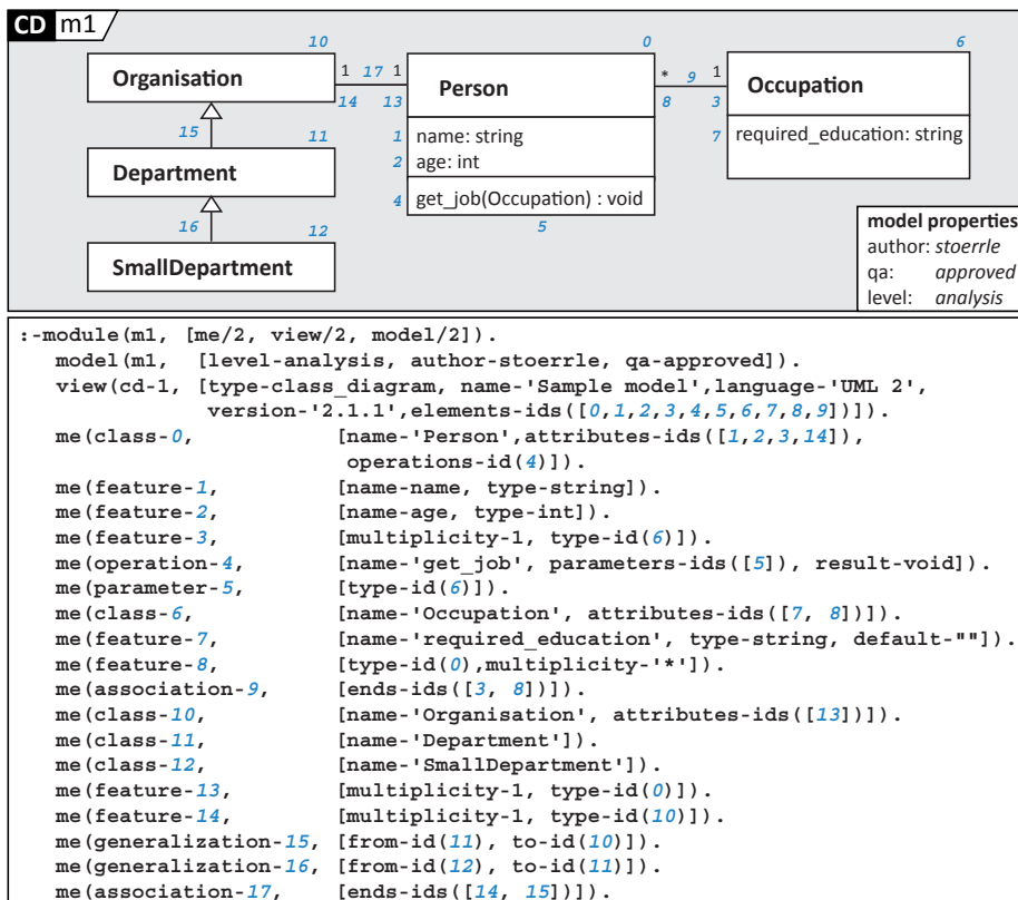
Figure 5: A sample transformation from a model containing a UML class diagram (top) into a Prolog module with clauses for each model element (bottom). The extra numbers in the class diagram refer to the identifiers of the Prolog code.
